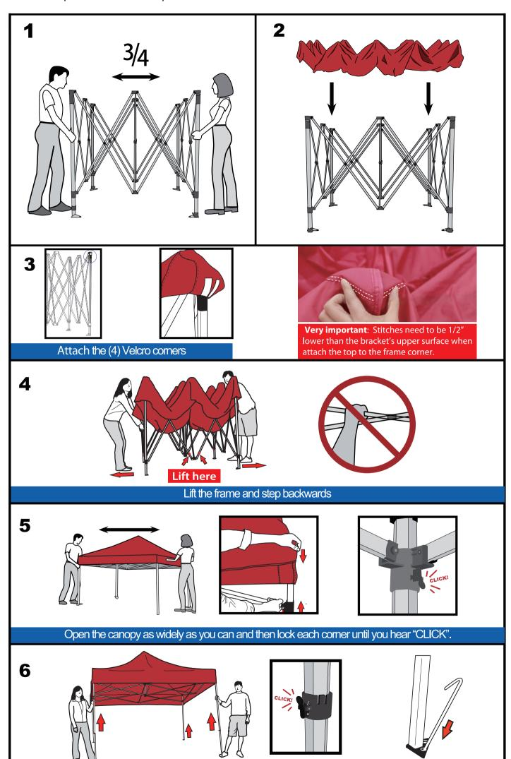
Step on footplate, pull leg upward until it locks in extended position.
