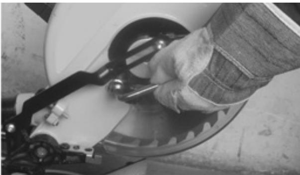
**Figure C: Removing Bolt**
