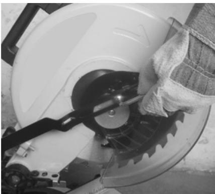
**Figure D: Removing Safety Screw**
