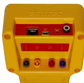
Tapered connectors best seal & easy release.
