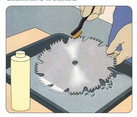
Clean the blade using a commercial resin solvent. (Commercial oven cleaner, turpentine, or a solution of hot water with ammonia may also be used.) For stubborn pitch and gum deposits, soak the blade in the cleaning agent in a shallow pan and use a brass-bristled brush to clean the teeth (above).
