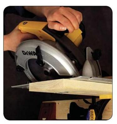
Even with its blade tilted to create a bevel, this 7¼inch circular saw cuts deep to saw through 1-inchthick stock.
