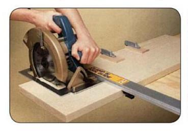
Some commercial guides can be extended up to 8 feet. The one shown at left is more suitable for crosscutting. It features clamps underneath the guide that secure the device to a workpiece, eliminating the need for separate clamps.
