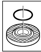
**Mounting flange for grinding spindle M 14:** An O-ring (plastic part) is inserted in the mounting flange 9 around the centring collar. **If the O-ring is missing or is damaged,** it must in all cases be replaced (article number 1 600 210 039) before the mounting flange 9 is mounted.
