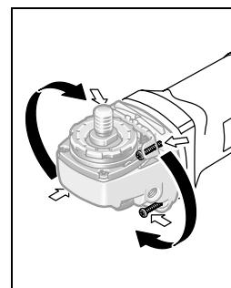
The machine head can be rotated with respect to the machine housing in 90° steps. In this manner, the On/Off switch can be brought into a more convenient position for special working situations, e.g. for left-handed persons.
