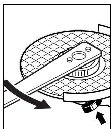
A properly attached, undamaged quick-clamping nut can be loosened by hand when turning the knurled ring in anti-clockwise direction.
