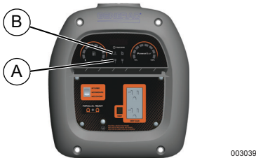
Figure 3-3. Shutdown Fault Generator Shut Down
