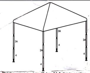
Slot the remaining legs (Tubes 3A & 4) into position ensuring the side tube holes are at the base. Push the plastic feet into place.
