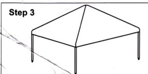
Assemble Gazebo cover, pull the cover tightly over the assembled roof frame.
