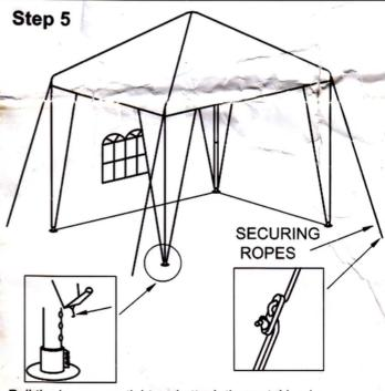
Pull the leg covers tight and attach the metal hooks into tube holes near the feet if the cover becomes loose, Tighten by moving the hook to a lower hole. The securing ropes can now be fitted if required.
