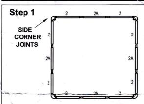
Assemble upper frame as shown using Tubes 2 & 2A and Side Corner Joints ensure that all poles are fully pushed into corner.
