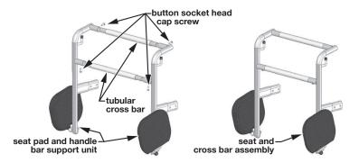
4. Insert the two tubular cross bars into the holes on the seat pad and handle bar support units as shown above. Align the small holes on the cross bar undersides with the holes in the support units. Install the four button socket head cap screws through the support units into the cross bars. Use the hex key to tighten. The finished assembly is shown at right above.
